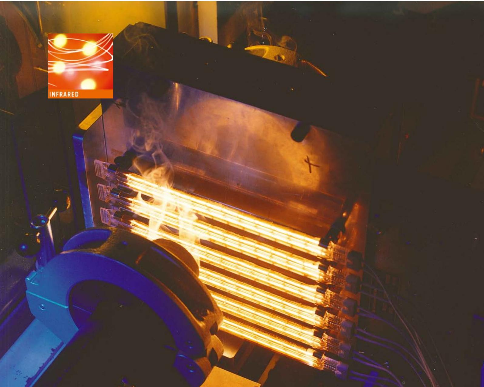
Infrared Systems for Plastic Welding
